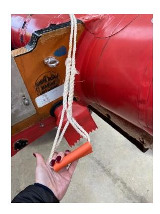
To check the rollover rope will not be entangled in the prop imitate the process of a rollover as shown in this picture \*\* Rope under the pontoon to check length of rope.
